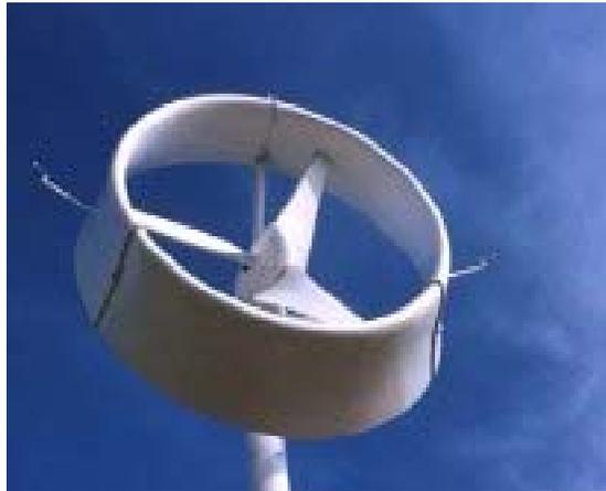
The performance of this technology has been verified in wind tunnel tests, and now TurbodynamX is seeking to validate this performance in the real world. Through several grants, the Illinois Institute of Technology has purchased one of the company's two 12 kilowatt prototypes of this technology and is currently looking for a site to install the unit and demonstrate its effectiveness. As opposed to wind turbines that you may
